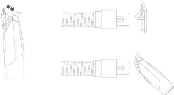
Before installing the knife, pull the movable knife adjustment knob down. Vacuum the dirt from the blade and trimmer.
